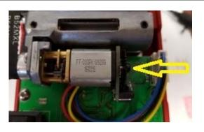
Step 4- Turn the power switch on while pressing the middle button. The motor should spin in fast speed for 10 min, (if the motor does not run, repeat step 3). When motor stopped, press the middle button again, the motor should reverse spin for 10 min. Repeat one more time spin each direction. Put the cover back.
