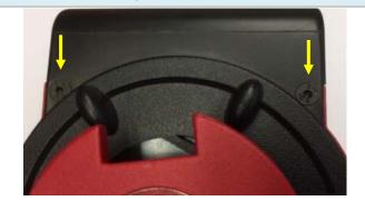
Step 2- Remove the screws on the top (2.5 mm hex key).
